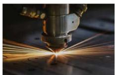
Laser cutting offers a high-quality cut and narrow kerf and can be used to cut aluminium, plain steel, stainless steel and spring steel.
