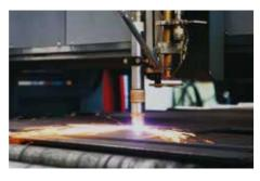
Plasma cutting is perfect for working on steel and non-ferrous materials that are under 254mm thick and its benefits include high levels of speed and accuracy.
